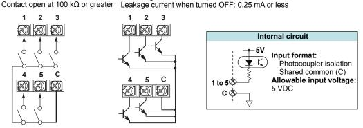
Dielectric strength: 500 VDC for one minute (between input terminals and the ground terminal)
